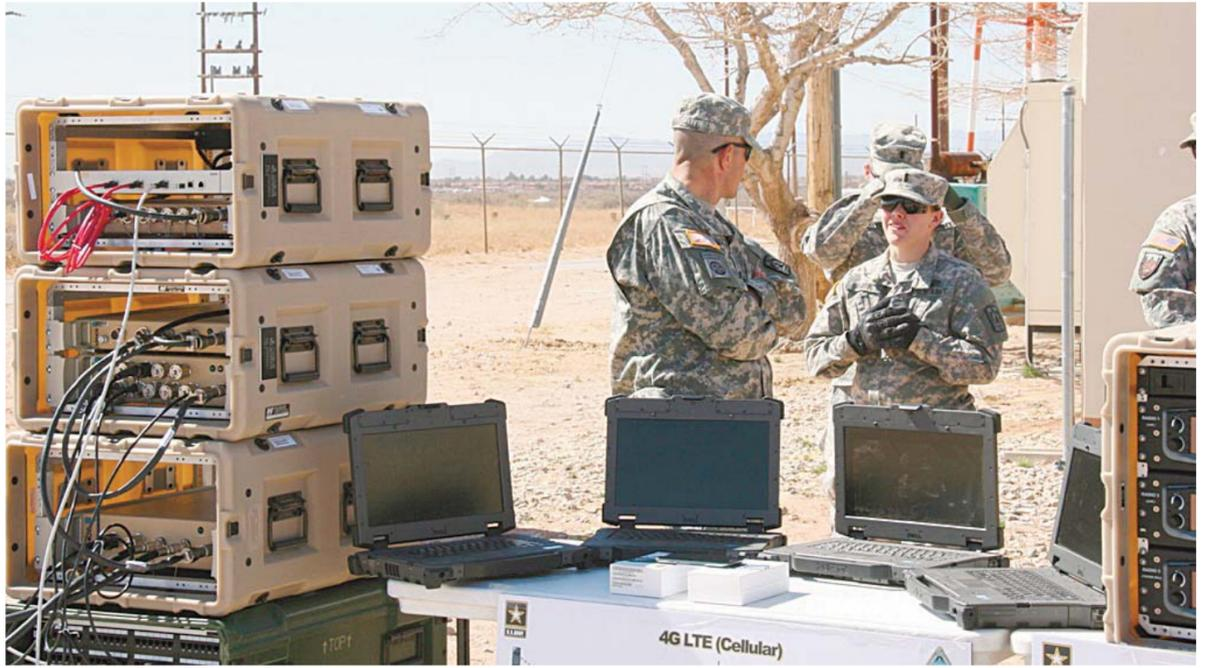
During Network Integration Evaluation (NIE) 14.2, the Army will evaluate a 4G LTE system that allows Soldiers to use the Secure Internet Protocol Router (SIPR) Network on the battlefield via mobile devices and Wi-Fi. The equipment shown was part of a demonstration for Warfighter Information Network-Tactical (WIN-T) Increment 1 advancements, at Fort Bliss, Texas.
